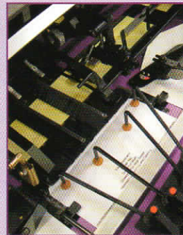
Machine vacuum control for positive envelope opening
